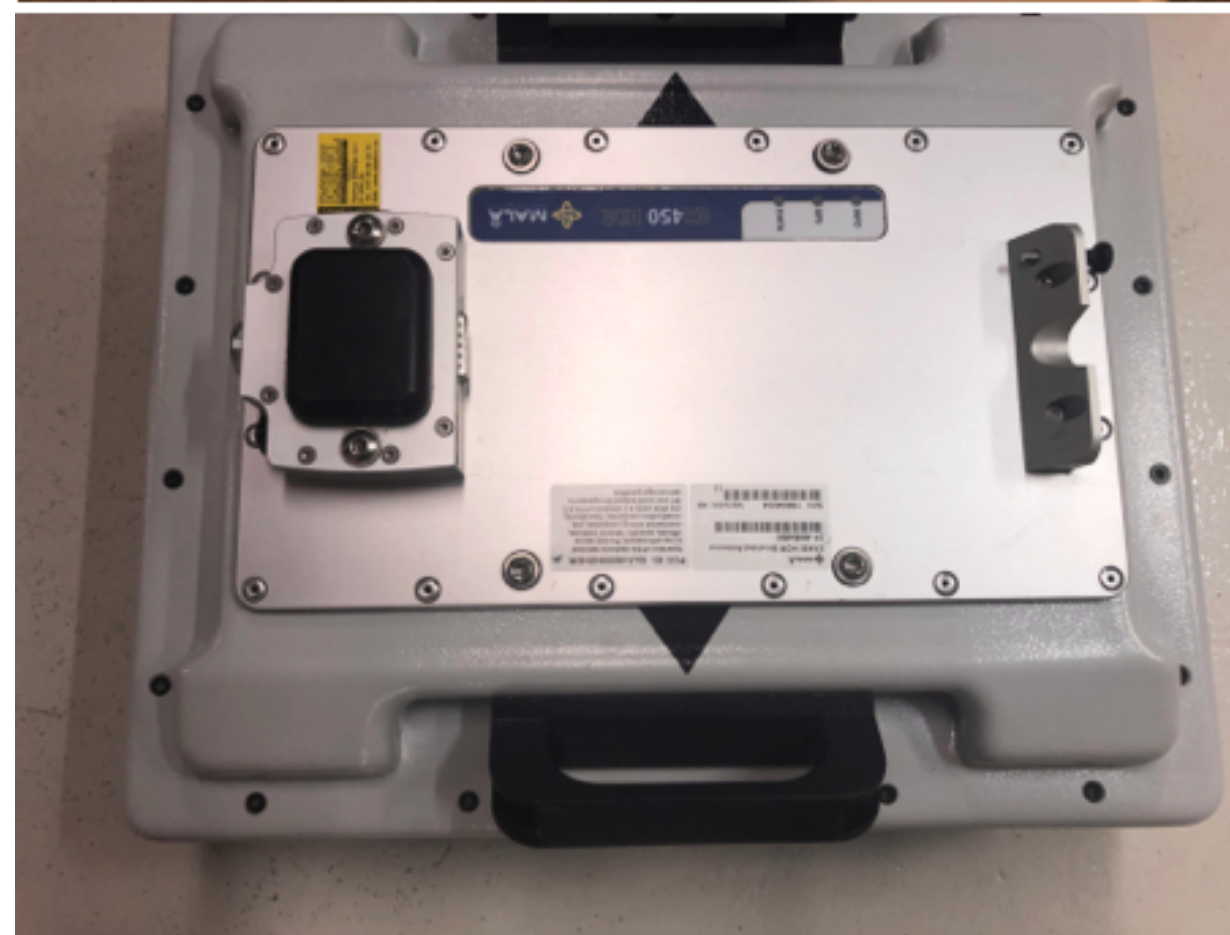
Antenna with transmitter and receiver
